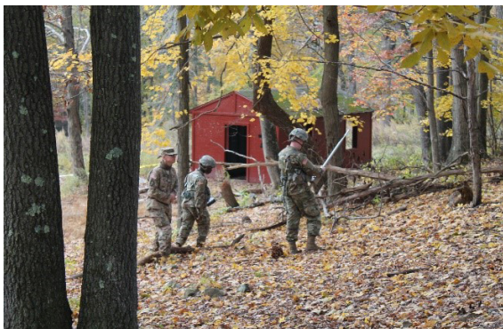
Figure 4. Cadet Nicholas Donze prepares to extend a telescoping survey meter to keep himself a safe distance from the high radiation area that a 1-curie source produces. Cadet Carlan Ivey trails with a handheld Geiger-Mueller counter to monitor the exposure rate.
